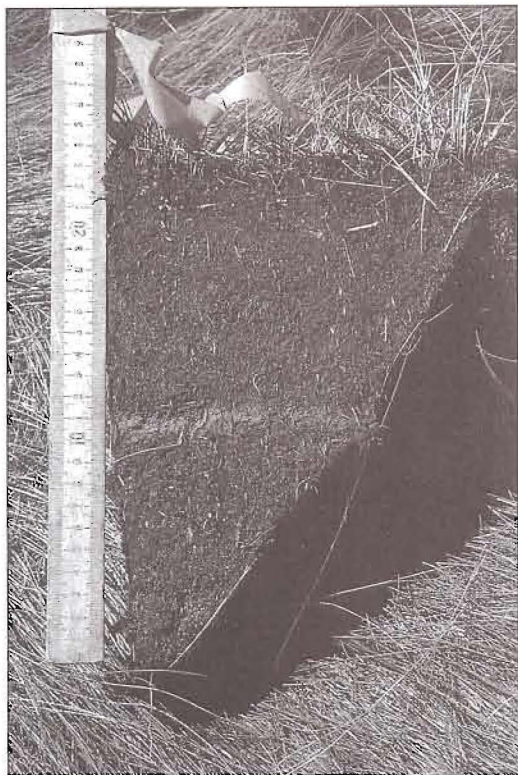
Fig. 2 A slice of peat from the Barn Island salt marsh which clearly shows a sand line 12-15 centimeters below the surface, produced by the 1938 hurricane. All the peat above the line has accumulated on the marsh since that date. (R.S. Warren)
